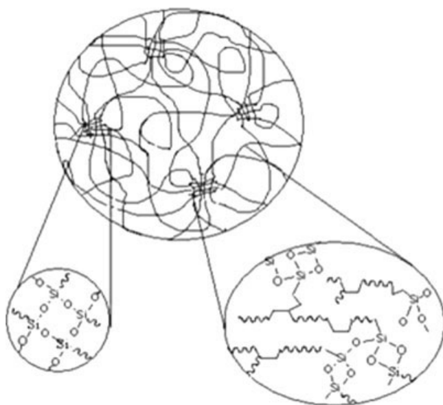
Scheme 2 A schematic model for UV-curing VTMS/AP hybrid films.
